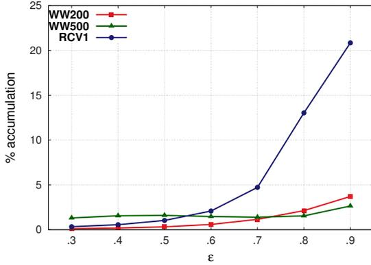
Figure 11: Mean percent accumulated non-zeros before pruning in pL2AP.
