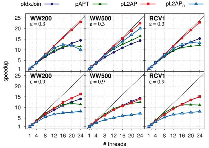
Figure 16: Strong scaling of parallel methods at  $\epsilon = 0.3$  (top) and  $\epsilon = 0.9$  (bottom).
