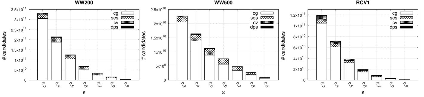
Figure 10: Pruning effectiveness in pL2AP. Each bar shows the number of candidates pruned during candidate generation (cg), at the onset of candidate verification (ses), during candidate verification (cv), and the number of candidates whose similarity was computed in full (dps), for  $\epsilon$  ranging between 0.3 and 0.9.
