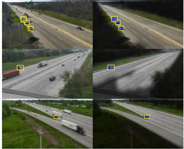
Figure 4. The traffic anomaly dataset containing traffic anomalies caused by vehicle crashes and stalled vehicles. The left column shows detected anomalies in the original frames. The right column presents background modeling results [26].
