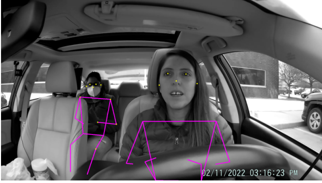
Figure 2. Human pose estimation for a frame of a video, showing detected key points and segments depicting major bones in the human body. Best viewed in color.
