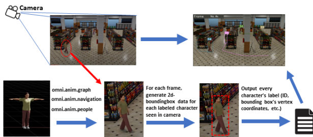
Figure 2: The framework of MTMC synthetic data generation. The Omniverse Replicator collects each character’s labels and converts them to a format usable by DNNs. The “omni.anim.people” extension is used to generate the scenario for each synthetic environment and enable each character to perform a sequence of movement.
